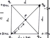
04. Calculate the Electric Potential at a Point P, Located at the Centre of the Square of Point Charge shown in the figure. [June2007]
